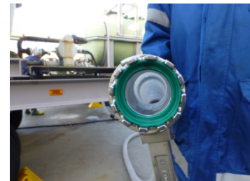
Open and cleaned hose
